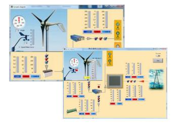
The Solar/Wind Energy Advanced Trainer is supplied with a software developed in LabVIEW that is able to communicate with the main components of the modular system via RS485 serial communication using Modbus RTU protocol, in order to perform a data acquisition and processing.
