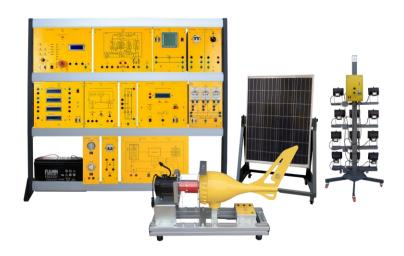
Modular trainer for the theoretical and practical study of the electrical installations with photovoltaic solar energy and wind energy.
