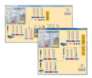
The ON-GRID solar energy with storage is supplied with a software developed in LabVIEW that communicates with the main components of the modular system via RS485 serial communication using Modbus RTU protocol to perform data acquisition and processing.
