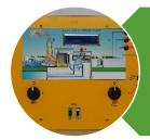
A power supply connected to the mains represents a coal plant connected to the infinite bus.
