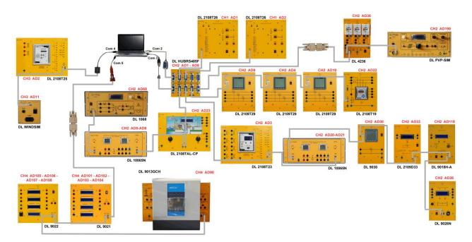
The SCADA project is divided in templates each one corresponding to a particular exercise. The open SCADA-WEB developers license provided with the trainer allows the teachers to fully customize the existing templates or create new ones that can be used to monitor the system from a local workstation.
