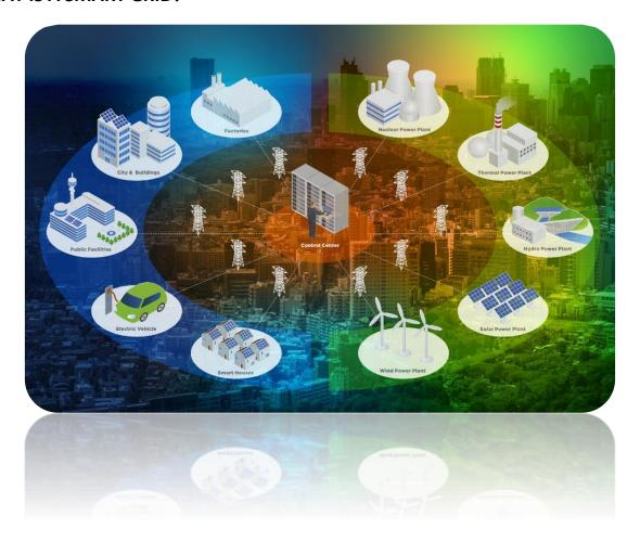
The Smart Grid is a system for an "intelligent distribution" of electricity, able to know the consumption of the various end users and to manage the generation and distribution of electricity according to demand.
