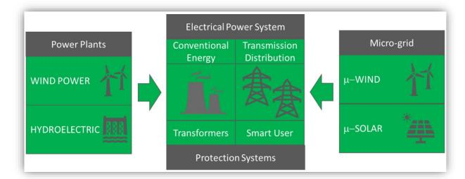
The smart grid system developed by De Lorenzo can be organized in **eight subsystems**, each comprised of several modules. The first four subsystems are simulations of energy sources; the first one is the main power supply of the grid with a three-phase supply unit that represents a coal plant.
