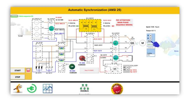
3. Increase the excitation voltage by pressing INC from SCADA, until the nominal voltage at the generator terminals (400Vac) is read on the digital measurement module.
