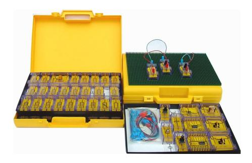
The kit includes a set of components allowing a full course on general electronics to be developed. All components are mounted on a printed circuit board fixed to metal tacks anchored on transparent plastic material modules, allowing consequently the vision of the components and the related symbol silk screened on the PCB, the mechanical protection of the component, the electrical safety against accidental contacts and easy replacement of damaged components.
