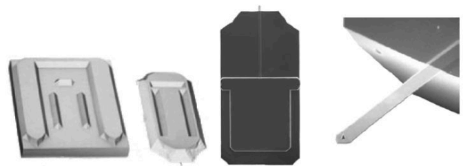
Figure 14: (Left) Alignment system. (Center) Cantilever chip viewed from the top. (Right) Cantilever, 450 µm wide with integrated tip.
