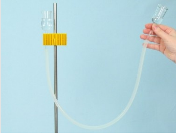
Water level with inclination of the bell
