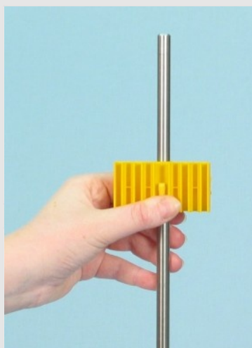
Fasten the glass tube holder to the stand rod
