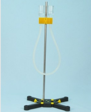
Comparison of the water levels of the experiment with the two glass bells
