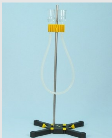
Test setup of the U-tube
