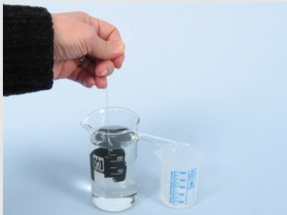
Overflow vessel with water and immersed irregular body
