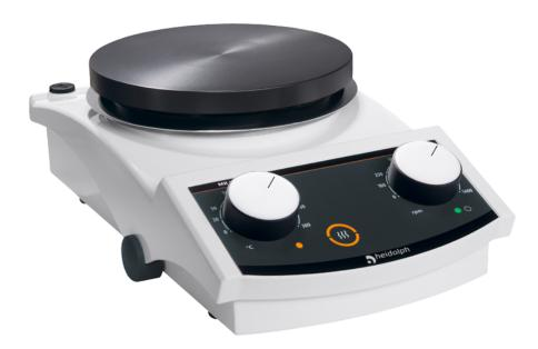
According to the motto "just stir and heat", our entry model of the Hei-Standard was manufactured with two rotary knobs to enable direct access to the two main functions. The speed and temperature are set using a scale. The maximum values are 1.400 rpm and 300 °C.
